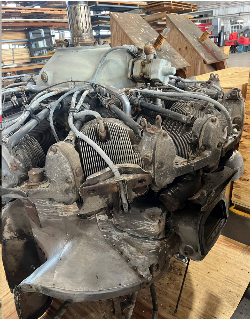
Removed from Lockheed C-60A aircraft: Engine, Wright R-1820-87, MFRS. NO. 157893
