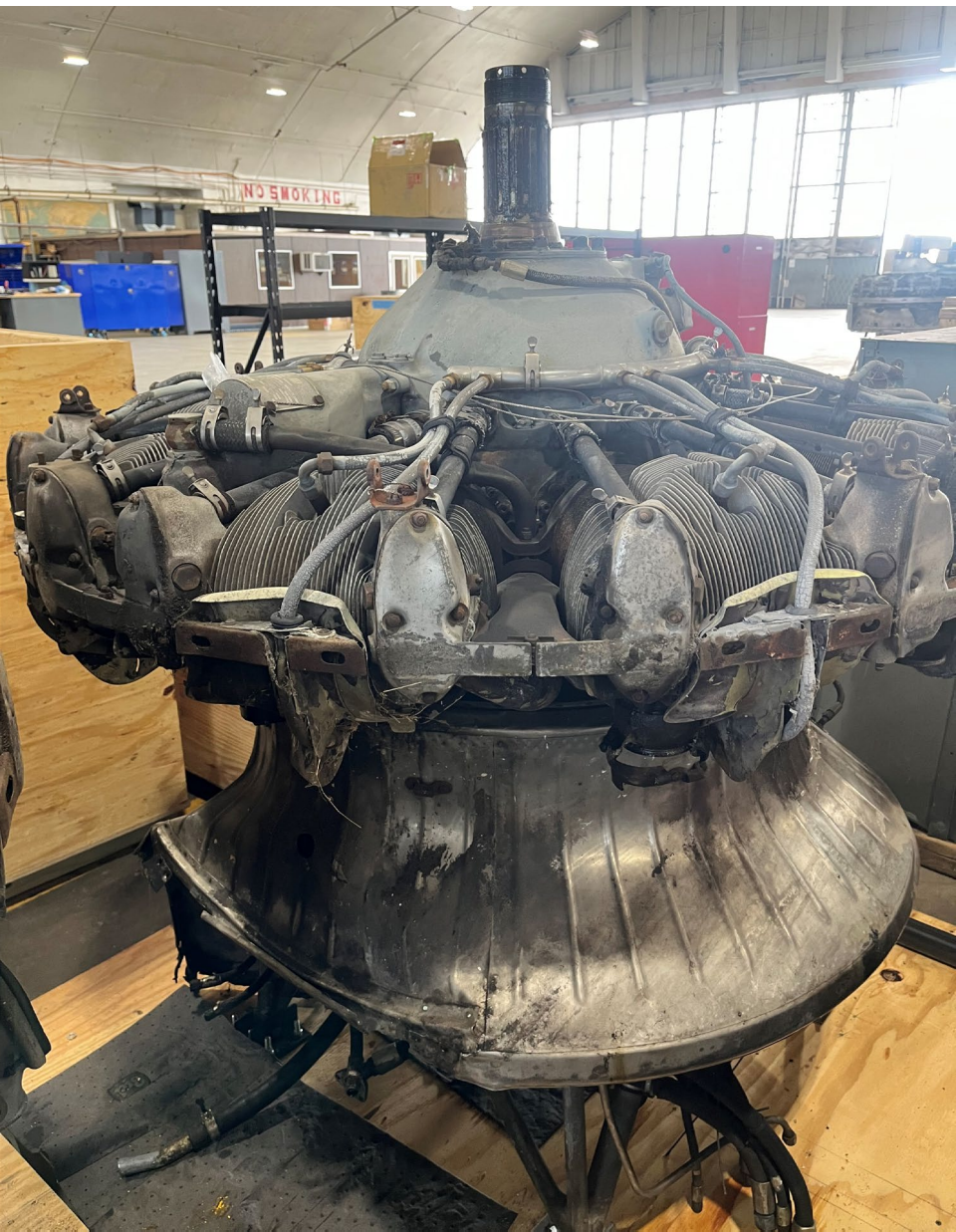
Removed from Lockheed C-60A aircraft: Engine, Wright R-1820-205A-87, MFRS. NO. 127546
