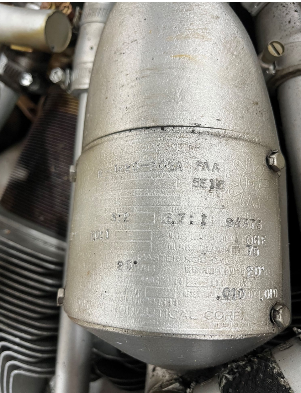
Removed from Northrop YC-125B aircraft: Engine, Wright R-1820-202A, MFRS. NO. 94373 (and propeller assembly)
