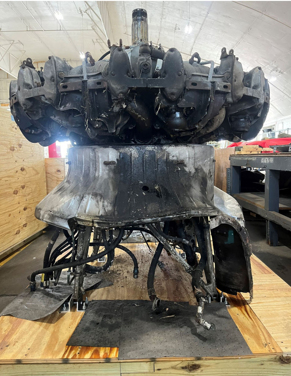
Removed from Lockheed C-60A aircraft: Engine, Wright R-1820-87, MFRS. NO. 157893
