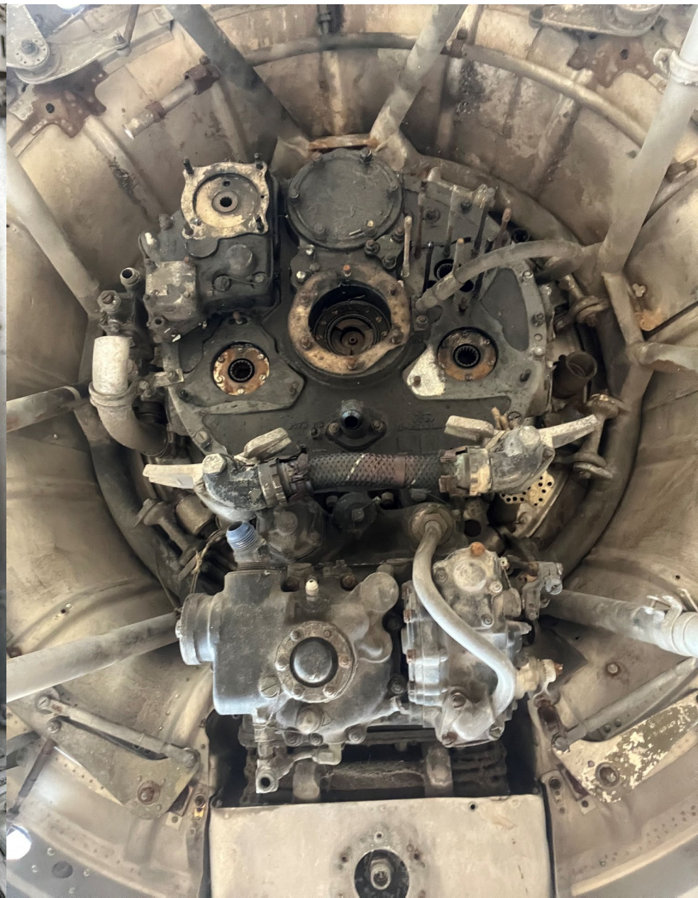
Removed from Northrop YC-125B aircraft: Engine Wright R-1820-97, MFRS. NO. SW-027805 (and propeller assembly)
