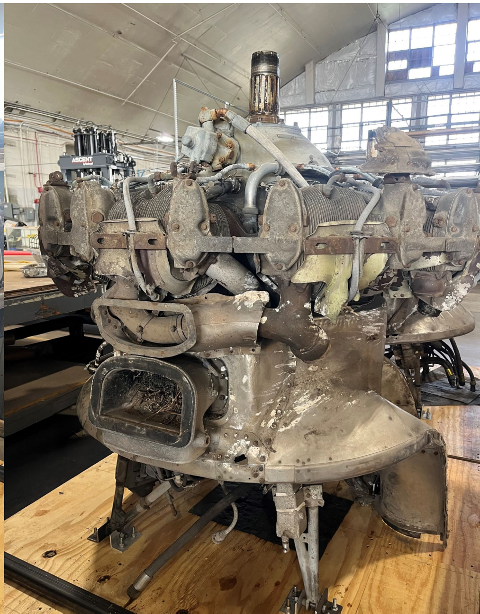
Removed from Lockheed C-60A aircraft: Engine, Wright R-1820-205A-87, MFRS. NO. 127546
